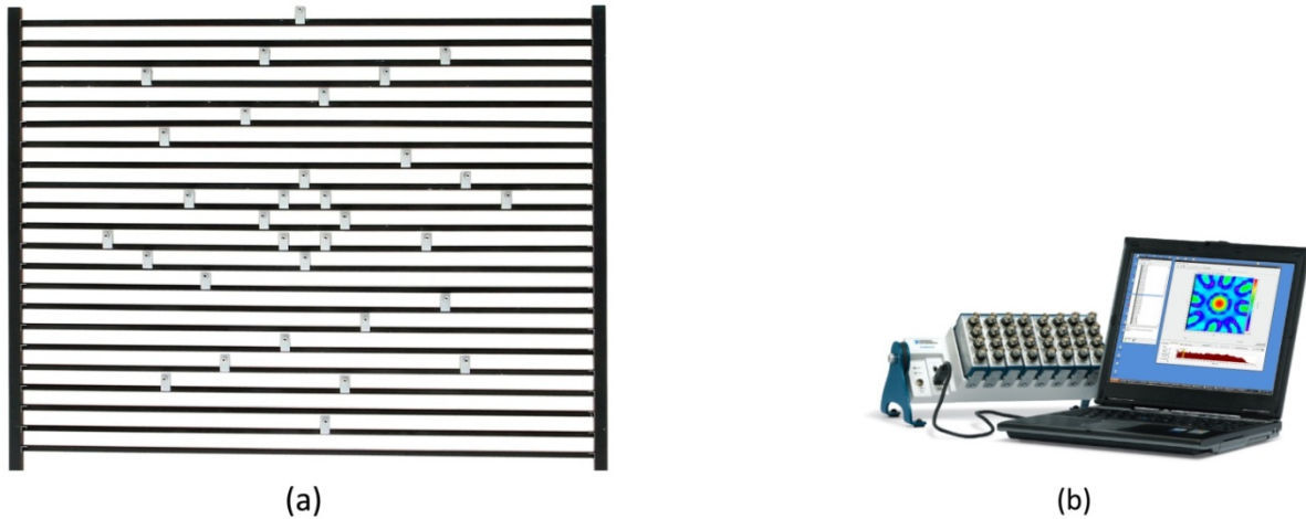
Figure 4. (a) Array of 32 microphones utilized; (b) Data acquisition system.
